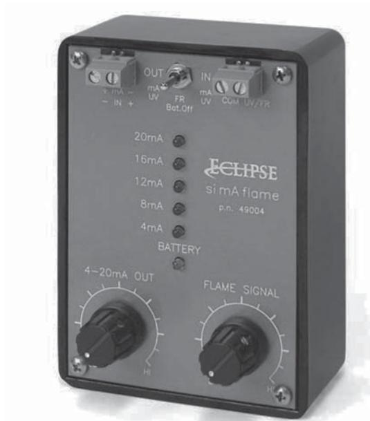
The Eclipse SimaFlame is a multifunctional tester that simulates flamerod or UV scanner flame signals to all major brand combustion safeguard controls. It also functions as a current loop checker. SimaFlame provides a variable 4-20mA output and can read 4-20mA inputs at five signal levels indicated by lights on the front face. These functions make this tool ideal for troubleshooting combustion control systems, including the temperature control loop.
